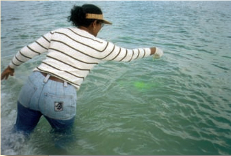
Measuring longshore currents with fluorescent dye.
