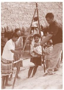
The A-frame used to locate contour lines
