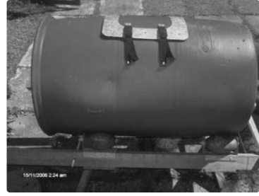
(b) Rotating tumbler composting
